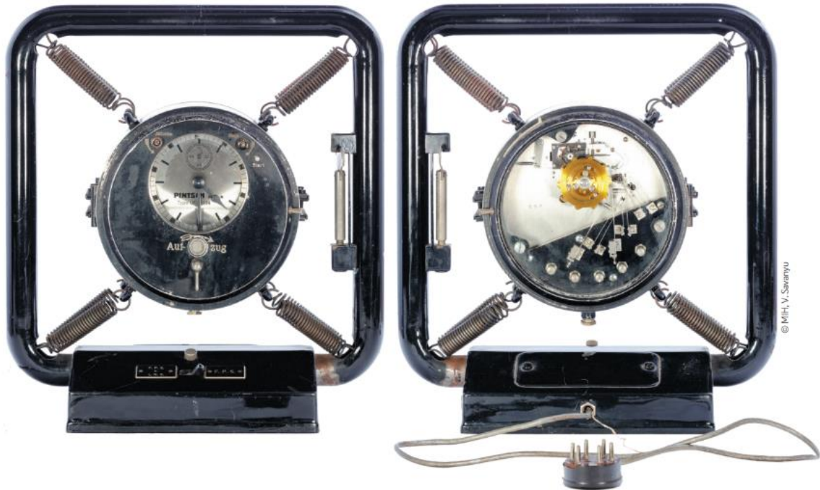
German Air Force signalling clock by Julius Pintsch, circa 1935 © MIH, V. Savanyu
